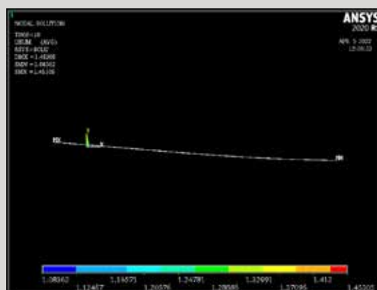
Ansys Mechanical model of the deformation of a 3-km natural gas pipeline subjected to multi-support excitation, simulating the effect of an earthquake for 10 seconds
