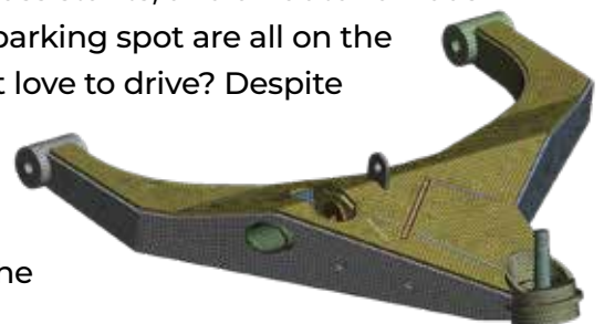
Lower control arm mesh in Ansys Mechanical
