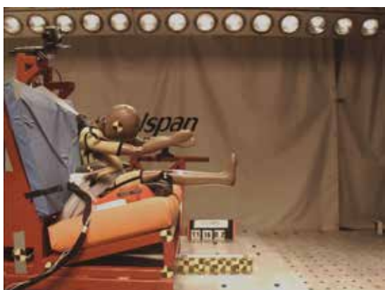
Physical testing using a crash dummy to verify simulation results
